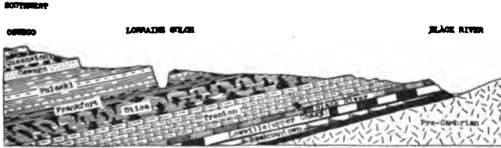
FIG. 1091. — Section southwestward from the Adirondacks and Black River to Oswego, New York, showing the relationships and succession of the Ordovician formations. Length of section about forty miles. Compare with section, Fig. 1057, p. 260. (Original.)
